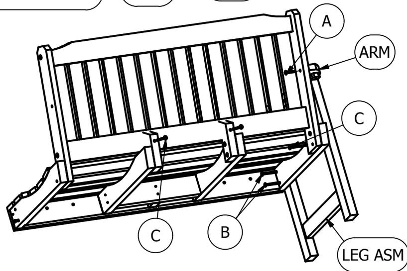
**3)** Attach Braces to Back Using Two "C" Bolts.
