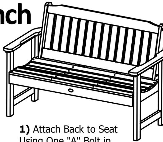
**1)** Attach Back to Seat Using One "A" Bolt in the Upper Hole on Each Side.
